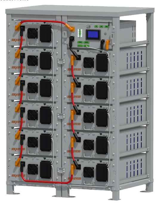
51.2V280Ah-HV high voltage lithium battery energy storage system, consisting of 8-17 battery modules (51.2V280Ah) and a BCU (Battery Control Unit) in series, with an operating voltage range of 358.4V-979.2V, is used for household / commercial energy storage applications, working with a high voltage inverter for energy storage purposes.
