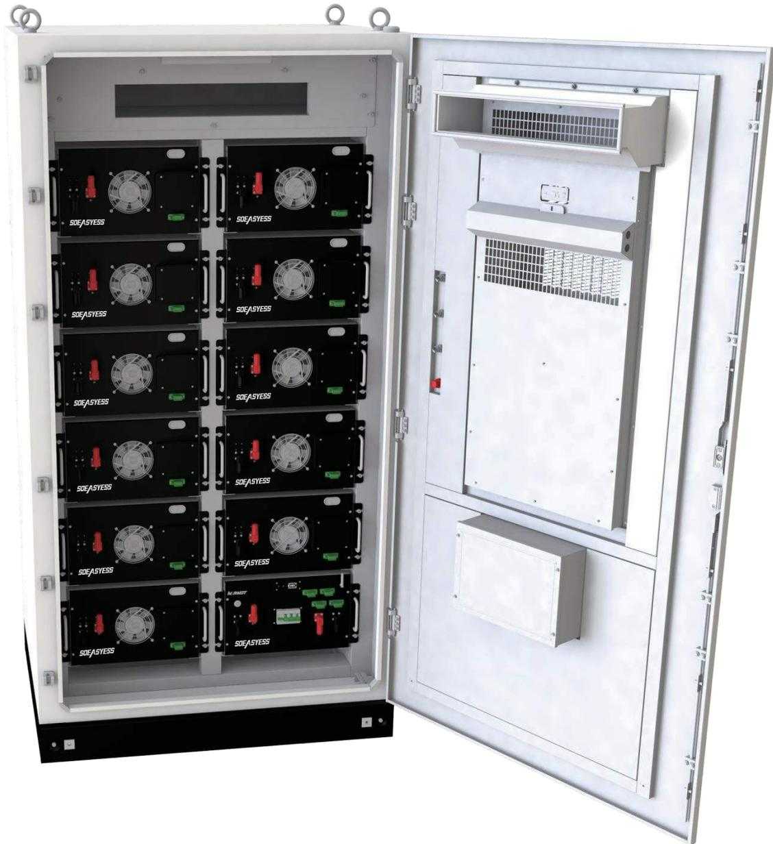
HV-51.2V200Ah high voltage lithium battery energy storage system, consisting of 6-11 battery modules (51.2V200Ah) and a BCU (Battery Control Unit) in series, with an operating voltage range of 185.6V-576V, is used for household / commercial energy storage applications, working with a high voltage inverter for energy storage purposes.
