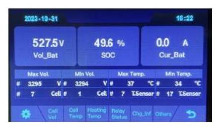
'Cell Vol': single cell voltage;
