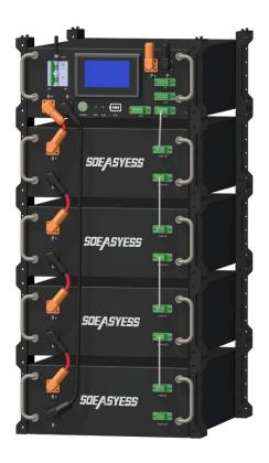
The high voltage lithium battery energy storage system consisting of multi battery modules (51.2V100Ah) and a BCU (Battery Control Unit) in series. Single set battery max. supports 17units, with an max. operating voltage range of 185.6V-980V, is used for household / commercial energy storage applications, working with a high voltage inverter for energy storage purposes.
